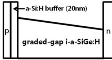
Figure 5. The schematic of a-SiGe:H p-i-n solar cell with a-Si:H buffer/graded-gap i-a-SiGe:H layer.
